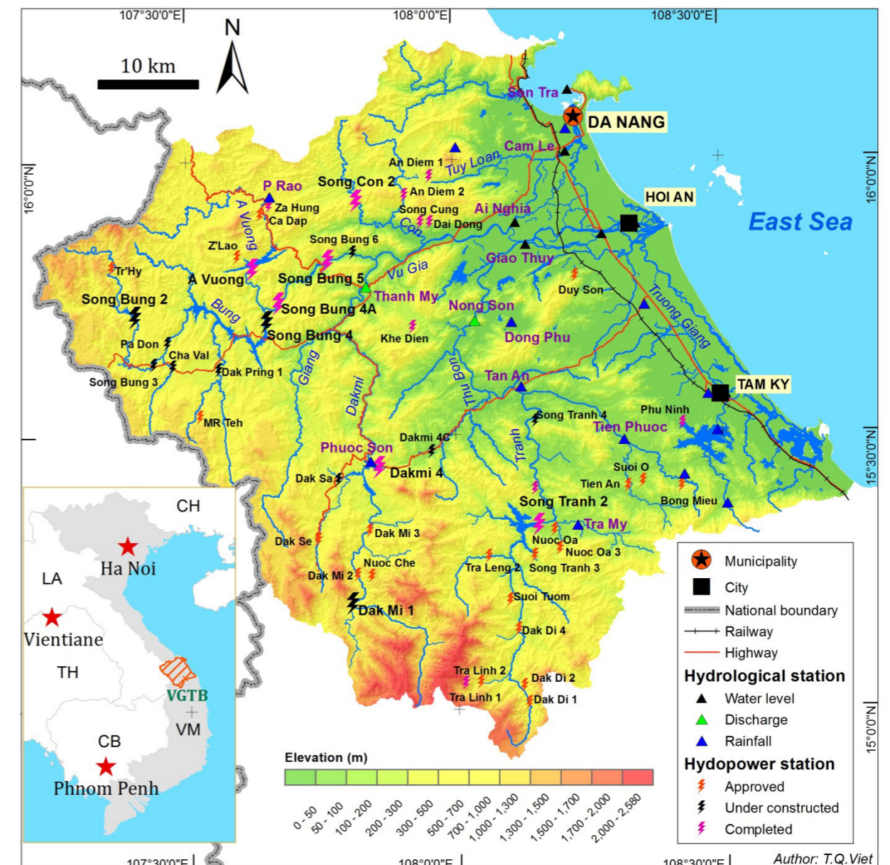
Figure 2. Sites of hydropower stations in the Vu Gia Thu Bon River Basin
